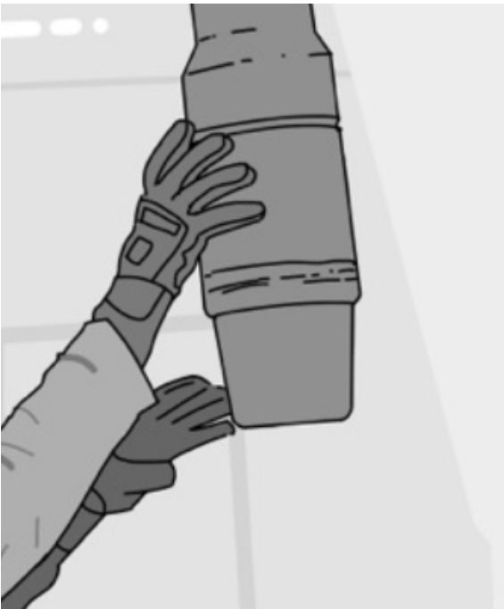
Thread Protectors on until connection make up
